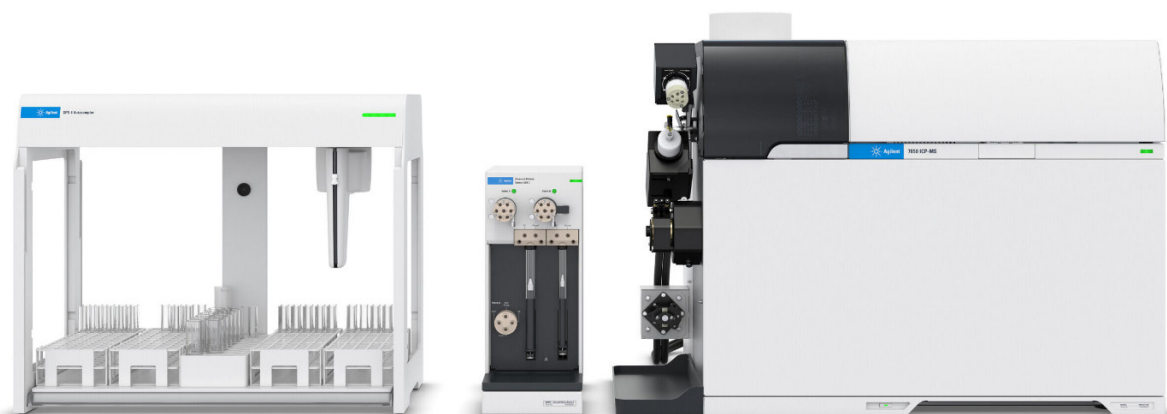
Figure 1. Agilent 7850 ICP-MS with integrated AVS MS (right), Agilent ADS 2 autodilutor (middle), and Agilent SPS 4 autosampler (left).
