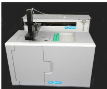
By utilising methods of cryotrapping and flow modification, it has been demonstrated that the system is capable of measuring small (sub 1ml) sample volumes and analysing DOC concentrations from 0.5 to 10ppm at levels of high precision (typically 0.1‰ for  $^{13}\text{C}$  determinations).
