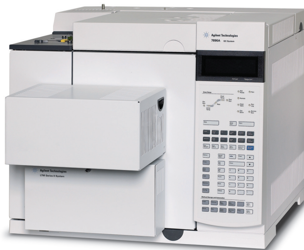
The Agilent 7890A GC equipped with the LTM Series II technology heats and cools the column very efficiently for significantly shorter analytical cycle times as compared to conventional air-bath GC oven techniques.
