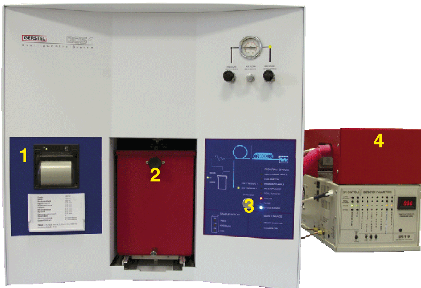
Figure 1. Quality Control System QCS 1 – Headspace Sampling System for beverage cans, in this configuration equipped with a Flame Ionization Detector FID; 1 optional printer, 2 sample oven, 3 control panel, 4 optional FID.
