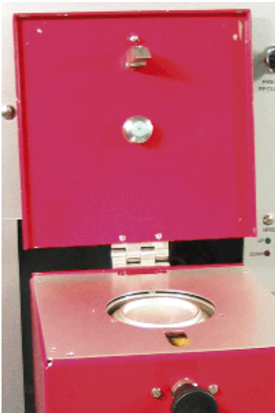
Figure 3. QCS 1 - Sample Oven for beverage cans. The picture shows the open oven with a beverage can inserted bottom-up. In the middle of the open oven lid a septum screw is seen. This septum screw presses the septum onto the convex bottom of the beverage can. Because of the conical shape the septum fits all type of beverage cans or other solid vessels. The extra hardened headspace needle penetrates the septum and the metal bottom of the can.
