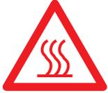
This warning sign denotes a hot surface, a high temperature hazard. It calls attention to a column heating block hotter than 70°C. For your safety, wear insulating gloves when the column oven is warm.
