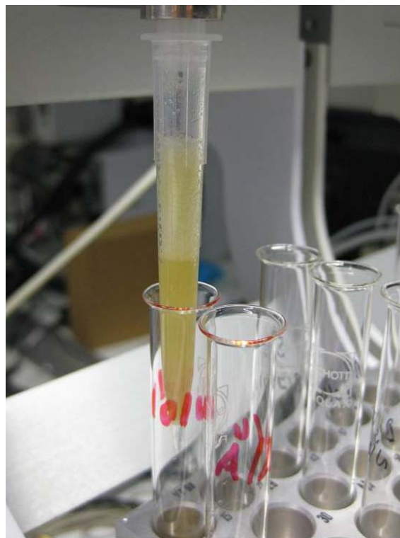
Figure 2. DPX extraction step. Turbulent mixing of sample and sorbent is achieved by aspirating air.
