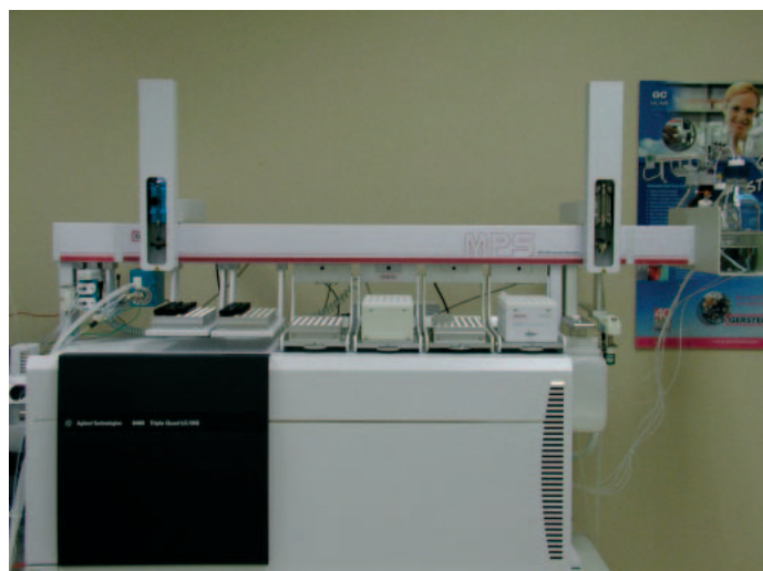
Figure 1. MultiPurpose Sampler (MPS XL) with GERSTEL DPX Option for high throughput barbiturates/COOH-THC screening.
