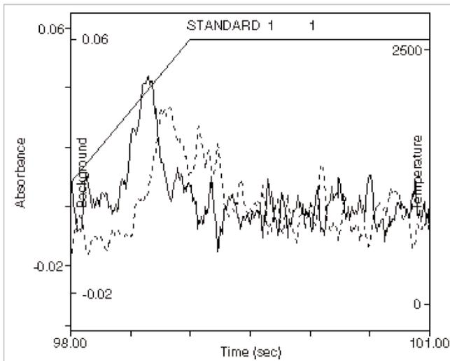
**Figure 4.** Typical graphic plot for selenium in serum with conventional R446 PM tube and normal hollow cathode lamp.
