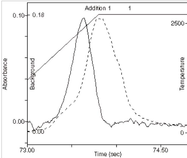
**Figure 3.** Typical graphic plot for selenium in serum with R166 PM tube and boosted discharge lamp.
