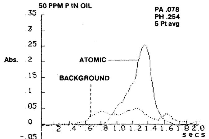
Figure 5. HP-85 Graphics printout CRA-90 Carbon rod atomizer.
