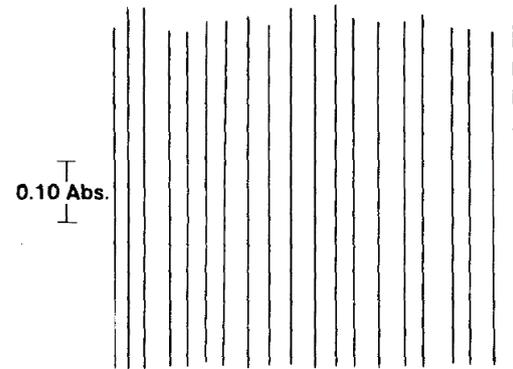
Figure 4. Reproducibility for phosphorus in oil CRA-90 Carbon rod atomizer.
