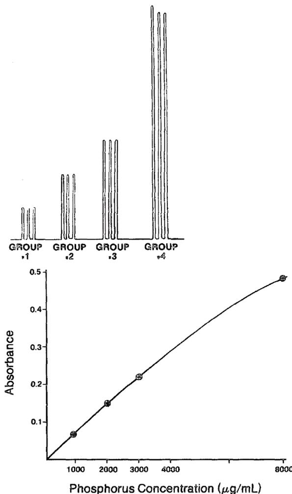
Figure 1. Flame determination of phosphorus in organic matrices.
