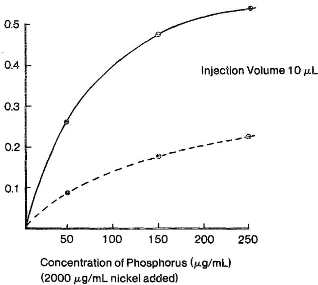
Figure 3. CRA-90 Determination of phosphorus in oil.
