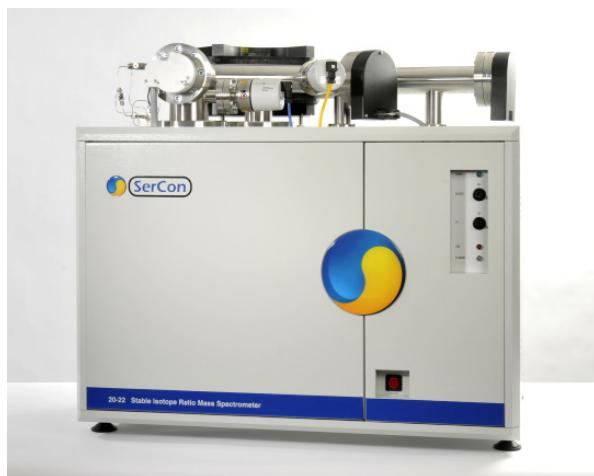
Sercon have successfully adapted their SL and GSL elemental analysers and 20-22 isotope ratio mass spectrometer to produce a system with the ability to perform this analysis.
