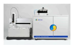
The Sercon heated sample bed can hold 220 samples in 5ml vials which are split into two halves that can be heated independently, meaning one set of up to 110 can be reacting whilst the other set can be being analysed resulting in high productivity.
