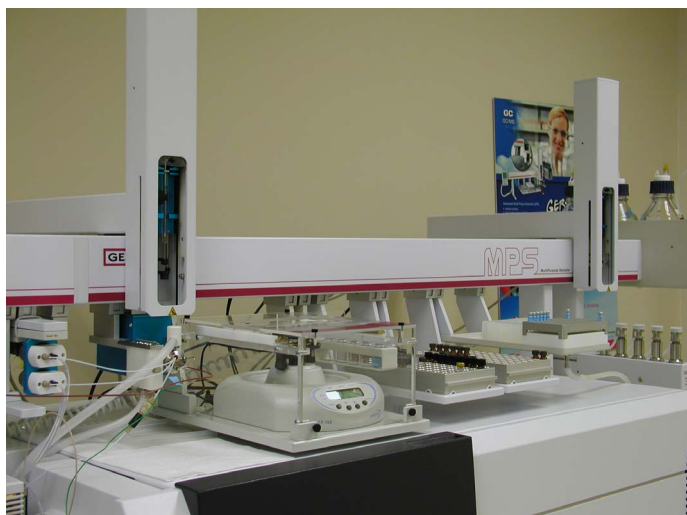
Figure 1. MultiPurpose Sampler (MPS XL) with CF-100 Centrifuge and ITSP Options.
