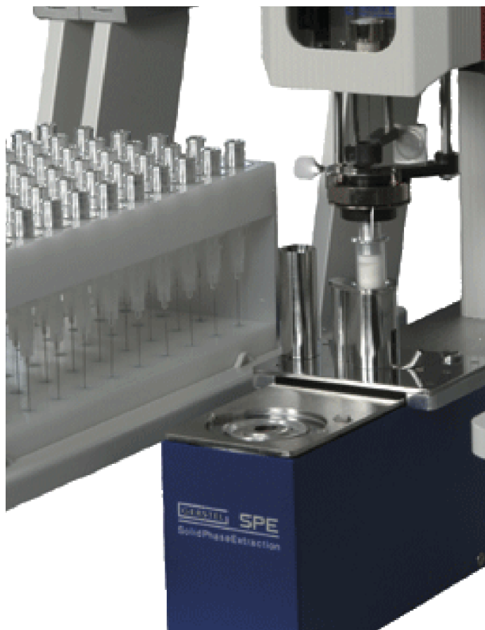
Figure 3. MPS SPE option with rack for 3 mL standard SPE cartridges (left) and elution unit with cartridge holder (right). The MPS is shown while transporting the cartridge to waste position. 1 mL, 3 mL and 6 mL standard cartridges can be used.
