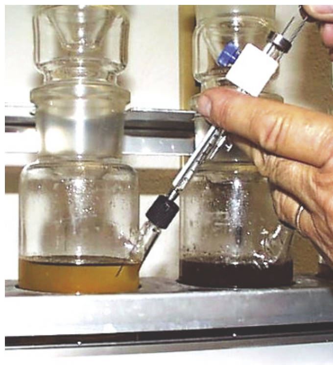
Figure 3. Taking a sample aliquot for GC analysis.
