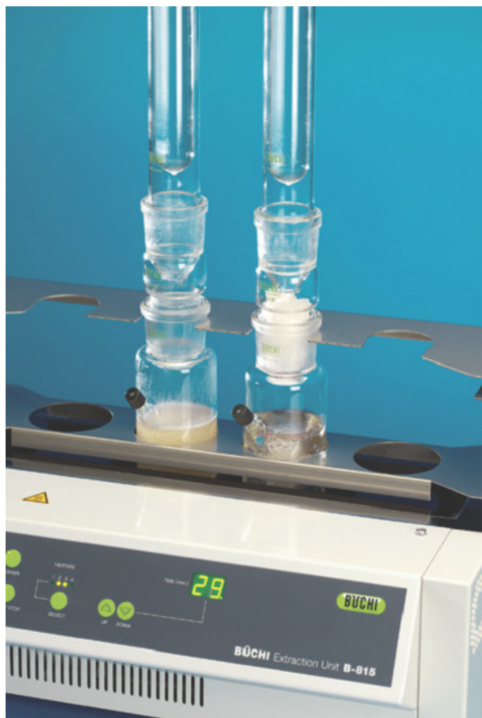
Figure 2. Simultaneous extraction and saponification in the Büchi B-815 Extraction Unit.
