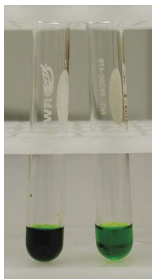
Figure 3. Photo of spinach extracts before and after dSPE clean-up.
