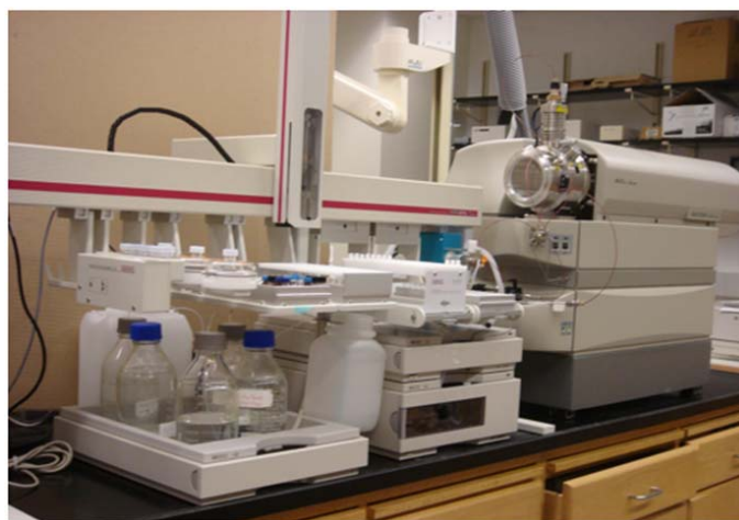
Figure 2. MPS 2XL MultiPurpose Sampler (MPS) with GERSTEL DPX option.
