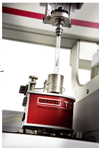
Figure 1. GERSTEL MultiPurpose Autosampler (MPS) with GERSTEL Thermal Desorption Unit (TDU) setup.
