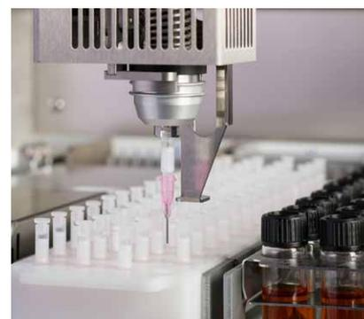
*Processing on FREESTYLE ThermELUTE™: Gripper with adapter takes the SMART column*
