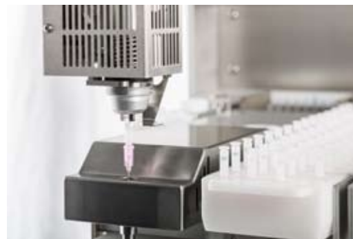
FREESTYLE ThermELUTE™ injects the eluate from SMART column directly into the HPLC
