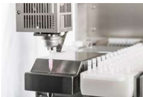
The immunoaffinity column OtaCLEAN is positioned into the ThermELUTE™ module.
