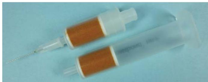
**Figure 2.** Top: Solid phase extraction cartridge configured for automated GERSTEL SPE. Bottom: Standard solid phase extraction cartridge.
