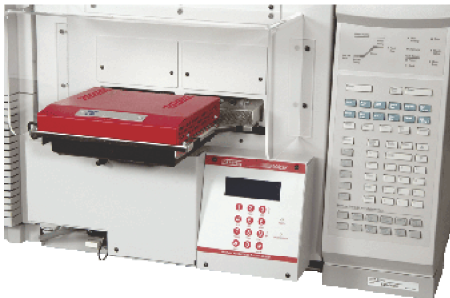
Figure 1. Single column MACH connected to 6890 GC system.
