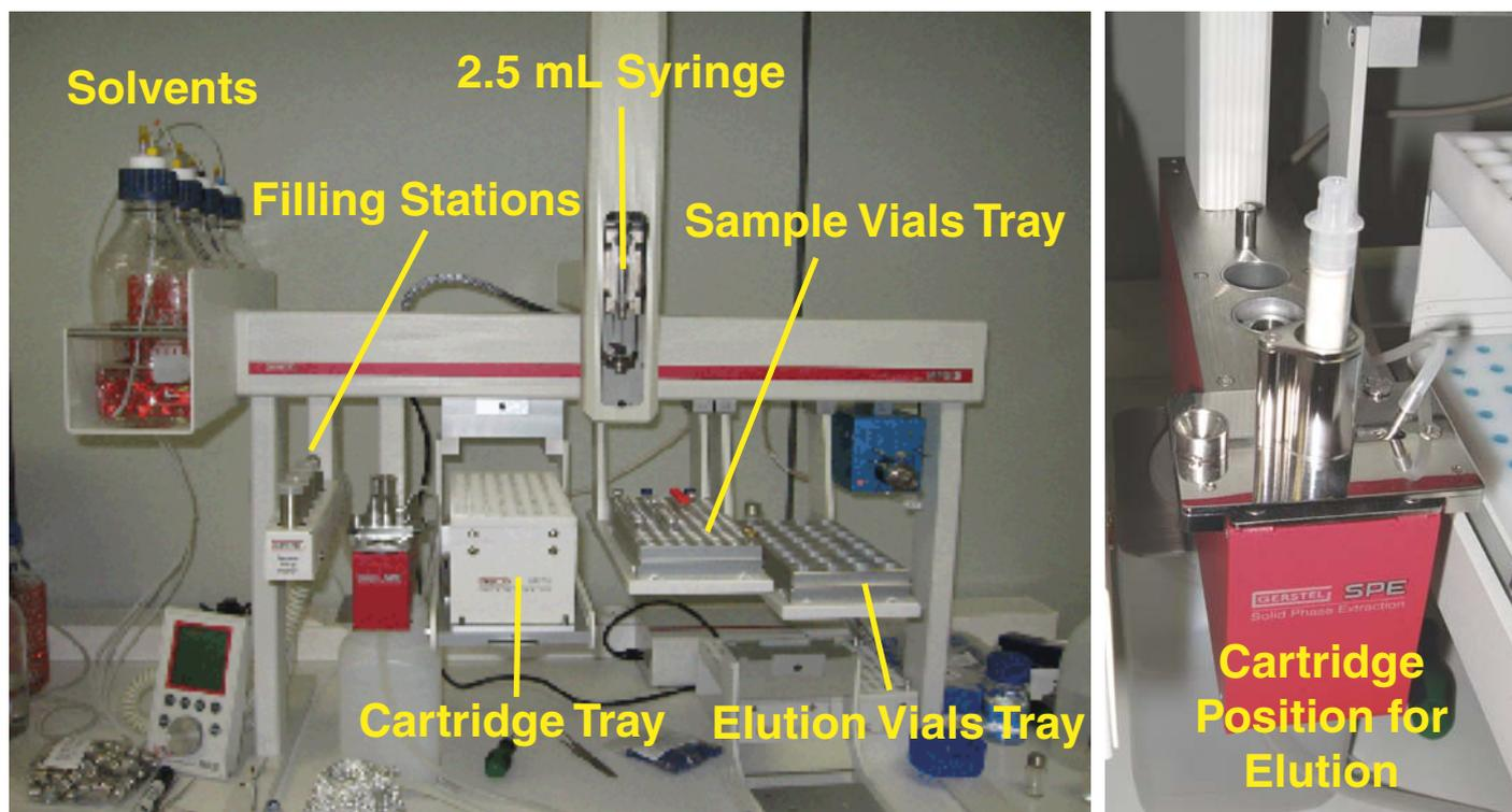
**Figure 1.** Gerstel MPS3 with integrated SPE option.
